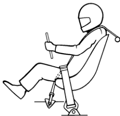
Figure 5: Safety Harness Mounting showing Correct Shoulder, Lap, and Crotch Strap Locations.
